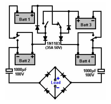
Here, Tesla has used four diodes to simplify the switching and reduce it to two On/Off switches plus two changeover switches. Alternatively, six On/Off switches can be used. As the diagram is a little difficult to follow when shown like that, the following diagrams may help by showing the current flow during the two states:
