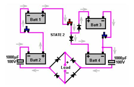
The State 2 wiring is almost identical, requiring another three On/Off switches and two diodes to avoid a permanent link between the plus terminals of batteries 3 and 4.
