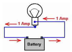
You will notice that the 1-amp current flowing out of the bulb is exactly the same as the 1-amp current flowing into the bulb. Exactly the same amount of current comes out of the bulb as the current which flows into the bulb. So, how much current is "used up" in doing the work of lighting the bulb? Answer: **None**. Energy is never destroyed, the most that can happen to it is that it gets converted from one form to another.
