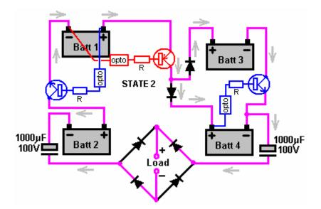
The suggested transistor switching for the State 2 situation is shown above. This is just an attempt to perform the switching with the most simple components available.
