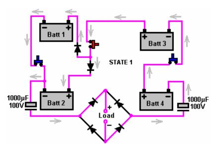
Here, batteries 1 and 2 are wired across each other while batteries 3 and 4 are wired in series. This needs three On/Off switches and the two diodes are inserted so that the plus terminal of battery 1 is not permanently connected to the plus terminal of battery 2, because in State 2, that connection must not be made.
