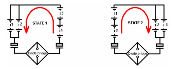
As you can see, this is essentially the same circuit with batteries 1 and 2 swapping over with batteries 3 and 4. But he has added in two capacitors and a diode bridge of four diodes to power the "load" (bulb, motor, TV or whatever). His circuit diagram is usually shown like this:
