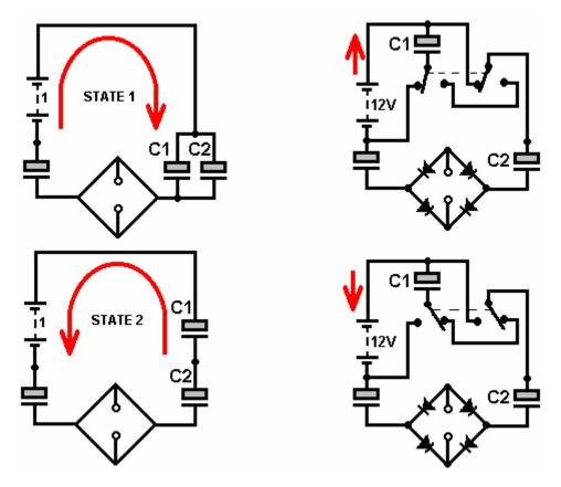
Here, two capacitors are used instead of two batteries. If the size of the capacitors is matched to the switching frequency, it should be possible to arrange it so that both capacitor C1 and Capacitor C2 reach the full battery voltage ('State 1' in the diagram) before the switch flips to the opposite state ('State 2' in the diagram). This then generates the reverse current cycle which is used to condition the battery.
