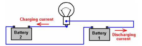
Here, the circuit is powered by battery 1 as before, but this time the current goes on to charge battery 2. Yes, battery 1 gets discharged just as before, but the plus side is that battery 2 is getting charged up all the time. The
