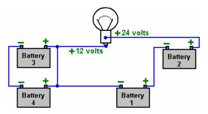
With 12-volt batteries as shown here, the bulb has the same 12 volts across it as it would have had with the single battery shown in the first diagram, as batteries 1 and 2 are wired "in series" to give 24 volts, while batteries 3 and 4 are wired "in parallel" to give 12 volts. Tesla arranged his circuit to swap the batteries over with 1 and 2 taking the place of 3 and 4. He chose to do it in a slightly different way and he swapped the batteries over hundreds of times per second.
