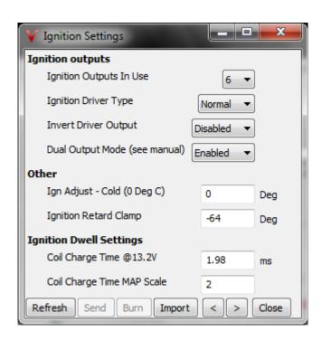
Set the dwell and number of ignition channels used on the Base Setup → Ignition settings menu.
