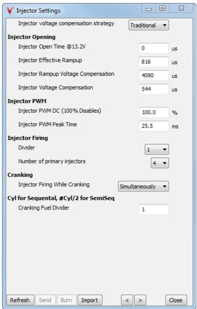
Choose the number of primary injectors, usually the number of cylinders. Divider is usually 1. For high impedance injectors, PWM DC should be 100% and Peak Time should be 25.5ms.
