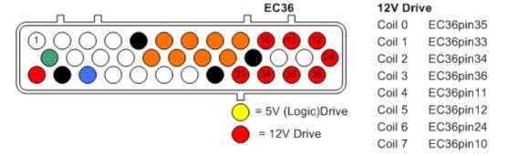
Option 0 All 8 ignition channels are using logic level(+5v) control for coils that have built in igniters or systems where you wish to use an existing igniter pack:
