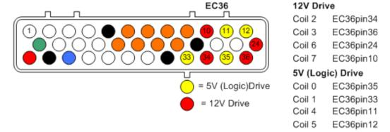
Option 6+2 Six high current channels, two logic level:
