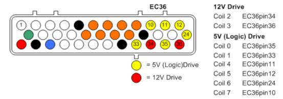
Option 4+4 Four high current channels, Four logic level:
