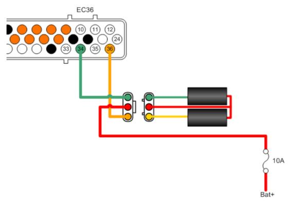
Additional coil packs, for applications such as 8 cylinder wasted spark
