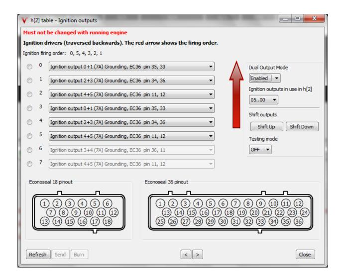
If you have a coil on plug or coil near plug coil setup, you can still run wastespark by enabling the Dual Output Mode. With this setting, each ignition entry will be two pins. You must make sure they are on opposing cylinders in the firing order.
