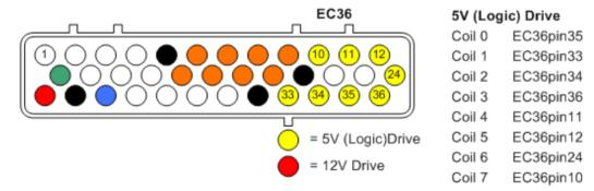
Option 2+6 Two channels are high current, the other 6 are logic level:
