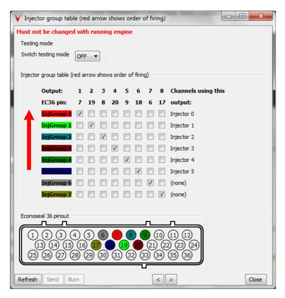
Setting the injectors like this will work fine, it's not important which injector fires when except for emissions. You can set the injectors to firing order, but it is generally recommended to wire up the injectors to the cylinder firing order. For instance, Injector 1 goes to the first cylinder that fires. Injector two goes to the second cylinder that fires.
