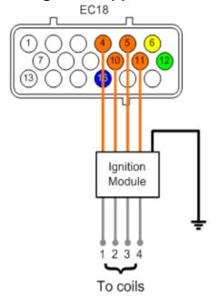
In some cases it has been found that we need to drive external ignition amplifiers (ignitors) using the higher current stepper motor driver.
